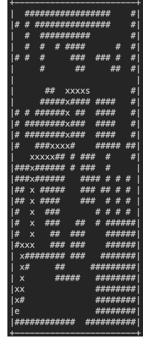
Fig. 3. A* algorithm running on a simulated "Dust II" map.
